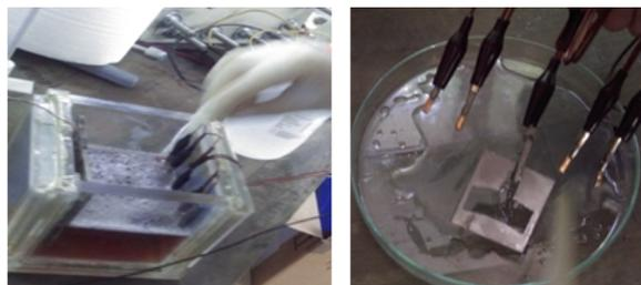
Fig. 1. The arrangement of 5 identical pieces in the electrolysis vessel (a) and their connection in a comb structure (b)
